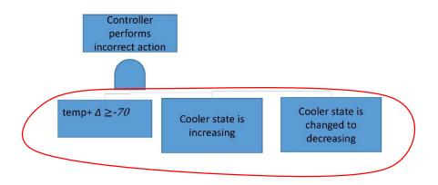
Always after controller reacted if sensor is OK and temp +  $\Delta \ge -70$  then cooler is in decr
