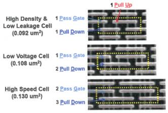
The picture shows three different memory cell layouts in Intel 22 nm FinFET technology.
