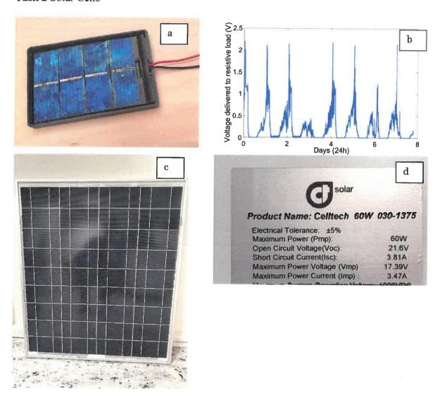
The pictures a)-d) show two different semiconductor based solar cells/panels. The small solar cell a) was characterized by connecting it to a suitable resistive load and a data logger.
