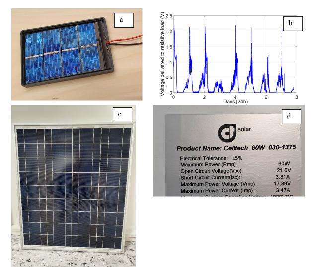
The pictures a)-d) show two different semiconductor based solar cells/panels. The small solar cell a) was characterized by connecting it to a suitable resistive load and a data logger.
