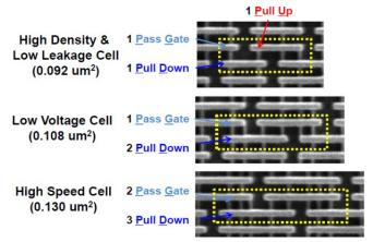
The picture shows three different memory cell layouts in Intel 22 nm FinFET technology.
