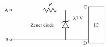
Assume that the integrated circuit (IC) in the figure above is fabricated using a relatively old generation of CMOS-technology with 3 nm gate oxide thickness.
