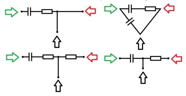
3. Based on the second observation from DC, we know that there is a capacitor because voltage over the resistor is increasing, and there is a resistor parallel to capacitor because voltage at the beginning that disappears over time. We can learn again total resistance:
