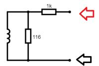
To calculate inductance based on time constant we need to know right resistance, which is R<sub>Th</sub>. In this case it will be short-circuited between Red and Black, so resistors are in parallel with R=1000//116=103.94 $\Omega$ . Since  $\tau=L/R$ , then  $L=\tau\cdot R=465\mu\cdot 103.94=48$ mH.
