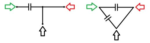
2. Based on the first observation with DC, there is a capacitor between Green and Red, because voltage over the resistor decreases. Since maximum value of observed voltage is 374.866mV, it means that there is an additional resistance. We can calculate this value as proportion between voltage over the resistor compared to total voltage with its total resistance:
