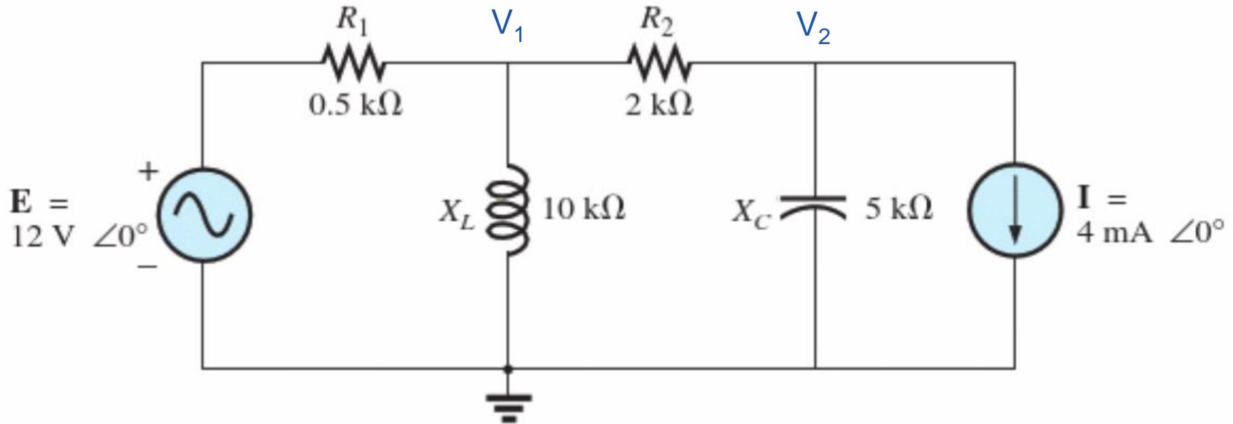
$$-\frac{V_1 - E}{R_1} - \frac{V_1}{Z_L} - \frac{V_1 - V_2}{R_2} = 0$$
