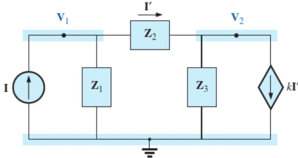
$$I - \frac{V_1}{Z_1} - \frac{V_1 - V_2}{Z_2} = 0$$
