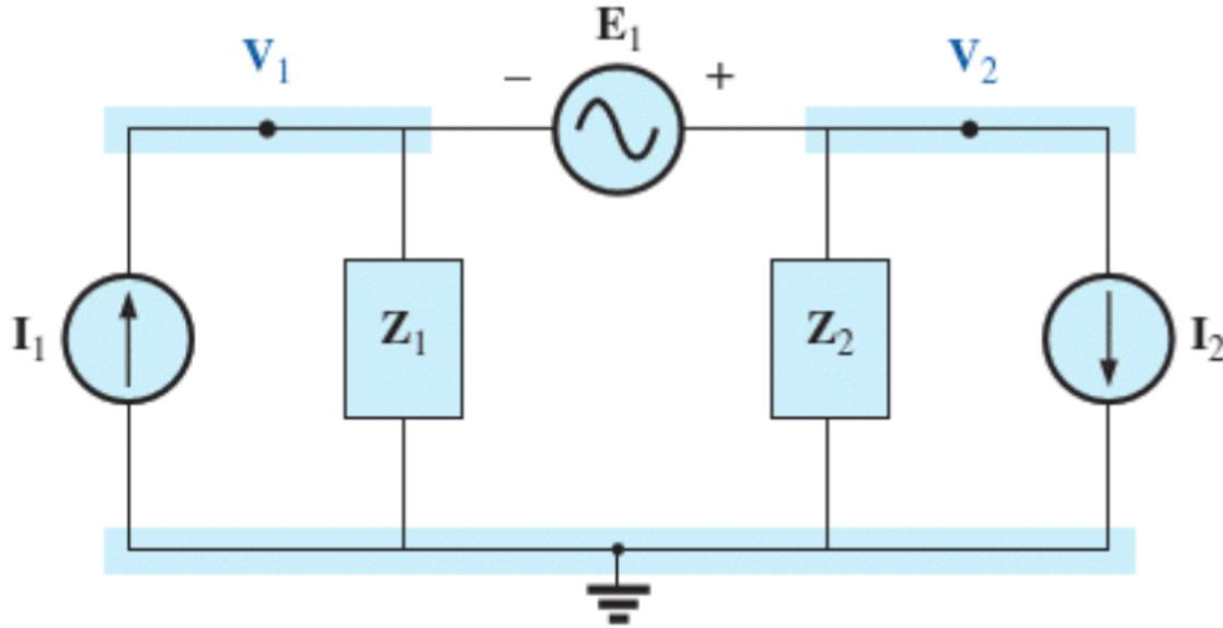
$$\text{Supernode: } V_2 - V_1 = E_1$$
