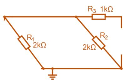
$$R_{\text{Th}} = R_1 // R_2 + R_1 = 2\text{k}\Omega$$
