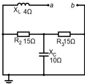
To calculate  $E_{Th}$ , we need to find a voltage on node **a** and node **b**. Since no current goes through the inductor, the voltage before the inductor is the same as voltage on node **a**. And it is equal to  $E_1$ . And voltage on node **b** is the same as  $E_2$ . Hence  $E_{Th}=220-100i=241.66\angle-24^\circ V$ .
