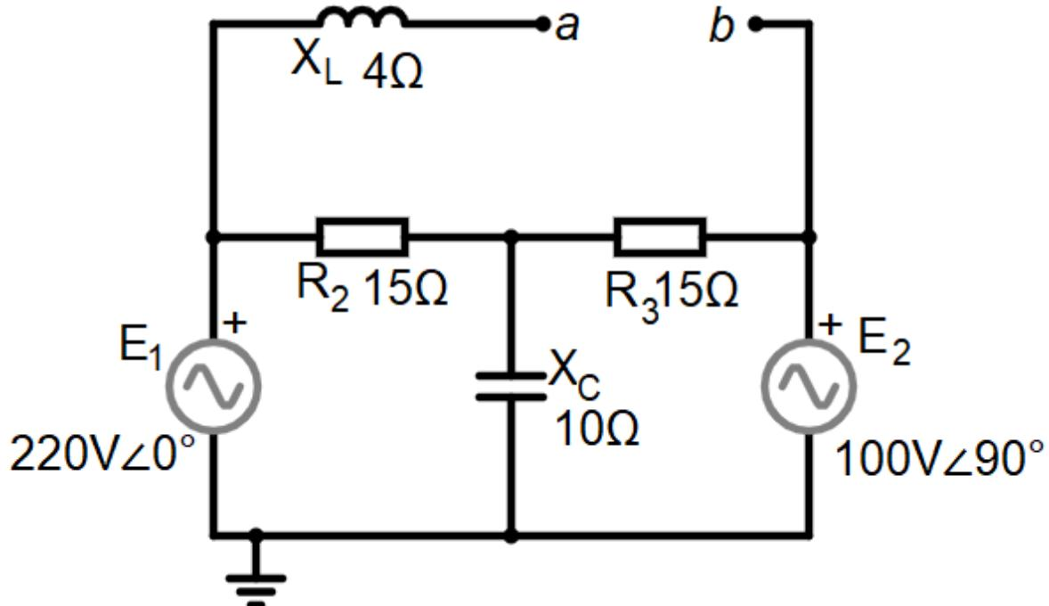
So first we are looking for  $R_{Th}$ . To do it, we remove voltage sources, then we see that  $R_2$ ,  $R_3$  and a capacitor are short-circuited, so we do not need to calculate them. So  $R_{Th}=Z_L=4\Omega$
