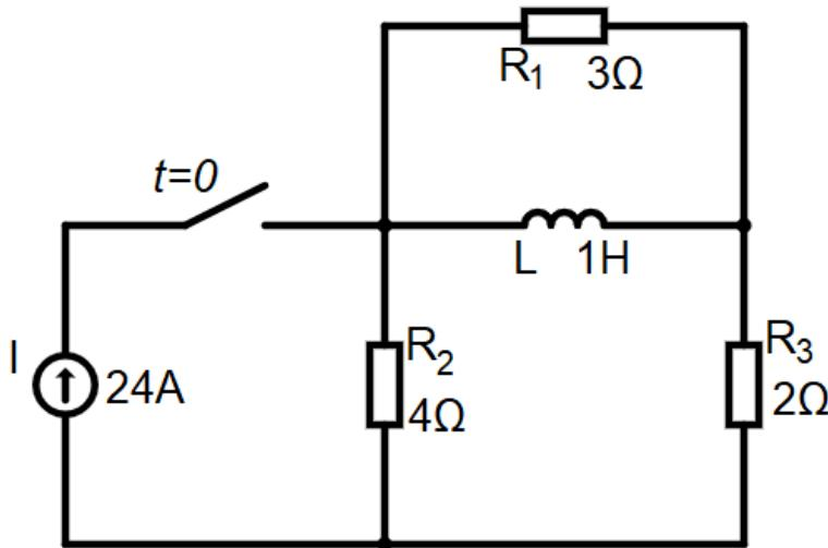
The circuit is too complex to solve as it is, and we need to find Thévenin equivalent circuit. We start by removing the inductor and determining  $R_{Th}$ .  $R_{Th} = R_1 // (R_2 + R_3) = 3 // (4 + 2) = 2$ . To find  $E_{Th}$ , we can convert current source to voltage source, with the value  $E = 24A * 4\Omega = 96V$ . Then  $E_{Th}$  is  $E - E_{R2} + E_{R3}$ :
